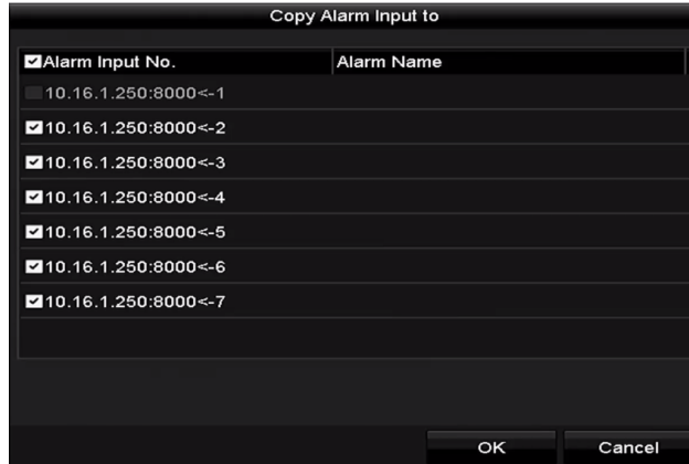
Figure 5-18 Copy Alarm Input
